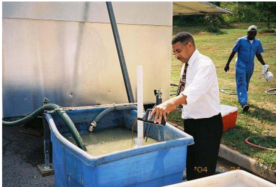
Figure 1: Adding motor oil to raw sewage. The mix of sewage, gasoline, motor oil, antifreeze (ethylene glycol), and a dandruff shampoo was then run through the RF-100 system.
